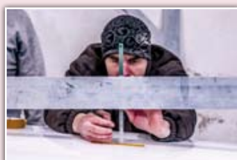
Marking offsets to keel with a ruler
