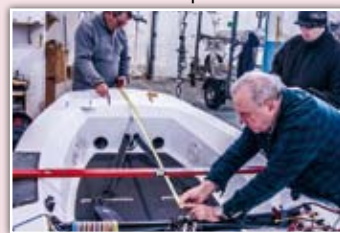
Measuring position of thwart
