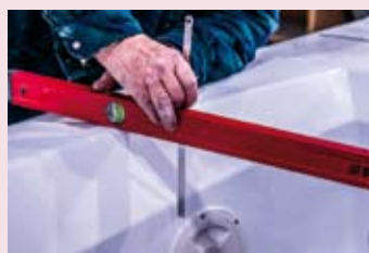
Measuring depth of cockpit
