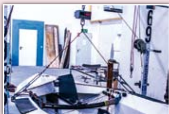
Hull is 110.8kg before correctors are added
