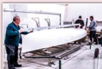
Fitting the strongback to create a baseline
