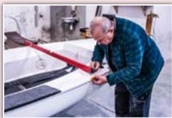
Measuring depth of cockpit at Station 2
