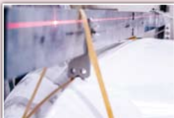
Levelling strongback with laser
