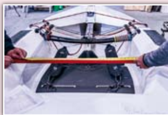
Measuring width of cockpit
