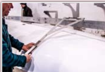
Marking stations on hull
