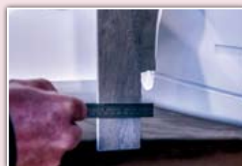
Station 0 showing tumblehome on template
