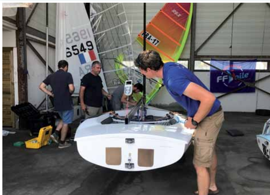
CHECKING THE MAST RAKE/TENSION, FOR CALIBRATING THE FIBRE OPTICS. BACKGROUND IN THE MIDDLE, PAUL IACHKINE, PhD IN SCIENCE AND TECHNOLOGY AND HEAD OF RESEARCH AT ENVSN IN QUIBERON.
